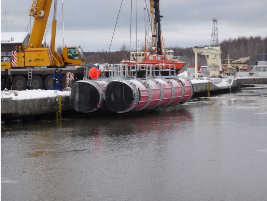
Figure 9. Towable tanks (“whales”) can be used for intermediate storage in the open sea and in the archipelago. Their capacity is 100 m 3 or 200 m 3 . © Jouko Pirttijärvi.
