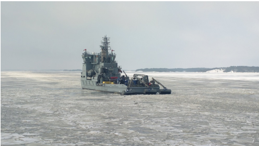
Figure 13. Ice oil brushes installed on the oil spill response vessel Louhi. The brushes have been developed by the Finnish Environment Institute. © Jouko Pirttijärvi.
