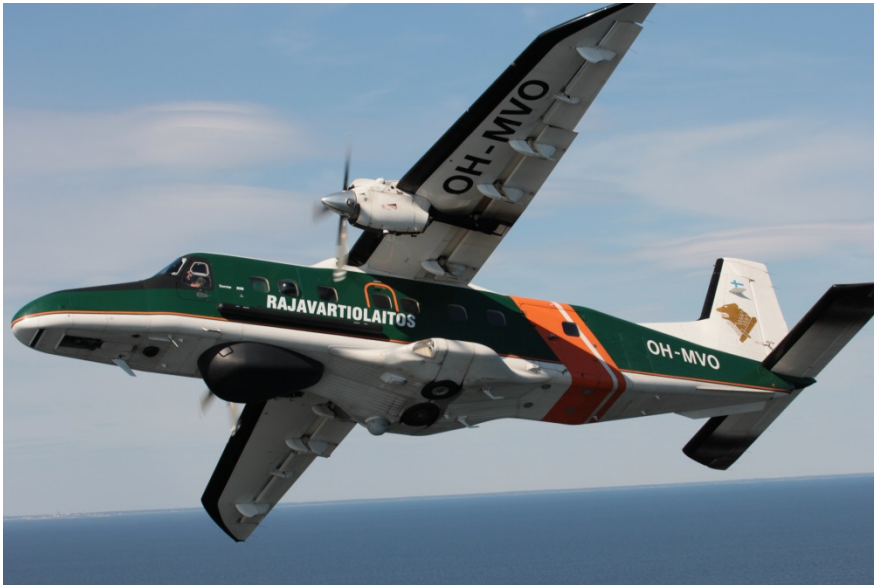
Figure 5. The Dornier Do-228 surveillance plane of the Finnish Border Guard has a range of 1,250 kilometres. © Finnish Border Guard.
