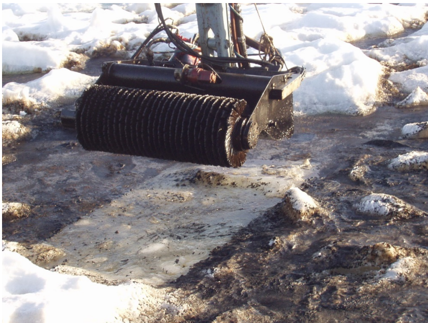
Figure 12. The brush recovery device installed in the bow crane of the response vessel Halli skims oil from the surface of the ice. © Jouko Pirttijärvi.
