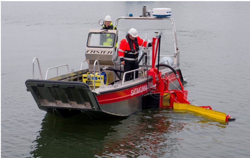
Figure 14. MiniBagger can be installed on all service boats with a length of more than six metres. The picture shows the newest boat of the Satakunta Regional Rescue Service. © Meritaito Ltd.
