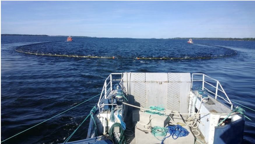
Figure 11. Gathering oil by means of seining. Auxiliary service vessels are towing an oil boom, while the oil recovery boat coming behind them is skimming the oil accumulating at the bottom of the boom through an opening at the bottom. © Jouko Pirttijärvi.
