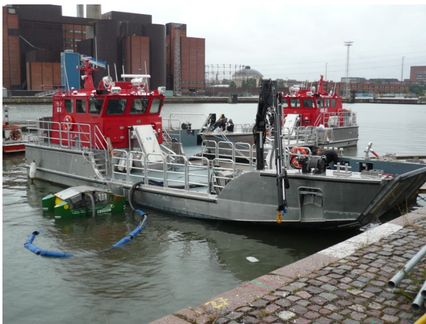
Figure 18. F-class oil spill response boat of the Helsinki City Rescue Department. The boat is equipped with integrated oil recovery systems. © Jouko Pirttijärvi.
